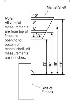
Figure 12 - Minimum Mantel Clearances for Built-In Installation
